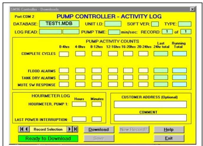
The retrieved information may be saved within the PC in a simple 'Microsoft Access' format for later analysis. ( The infrared receiver probe and software package are available as separate product, 'SM96 TERM', which also supports the SM97 Dual Pump version of the controller . )
