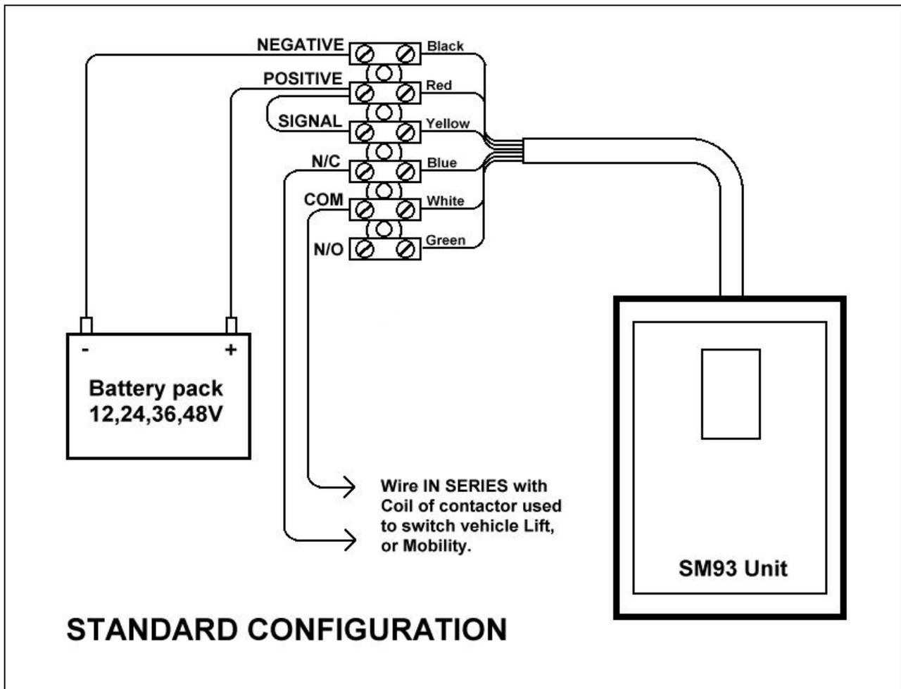
It is important that the **Positive** and **Negative** wires go *directly* to the battery. If the unit were to be wired simply to the nearest positive point in the dash or console, then voltage drops in the vehicle wiring loom could give artificially low voltage readings to the display when the wiring loom or vehicle is under load.
