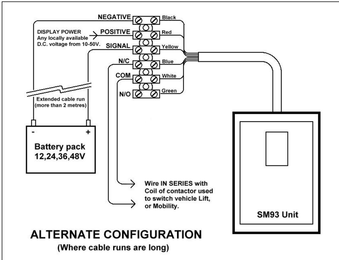
The Signal wire must be connected directly to the battery and the **Positive** wire can come from any nearby D.C. source ranging from **10V** to **50V** to power the display electronics. Where a local supply is unavailable, this **Positive** wire may be wired back to the battery on a separate conductor.
