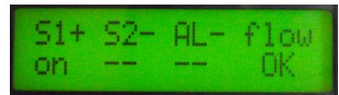
An adjustable timer (settable between zero and 200 seconds) will provide a 'wait' time after a High Level Alarm. It will inhibit the two output relays until there has been sufficient drain time in the sump tank. This prevents excessive cycling of output sprays & pumps.
