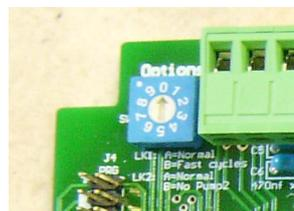
A small rotary switch on the controller backplane (shown left) may be rotated to one of ten positions to engage various display and functional test options.
