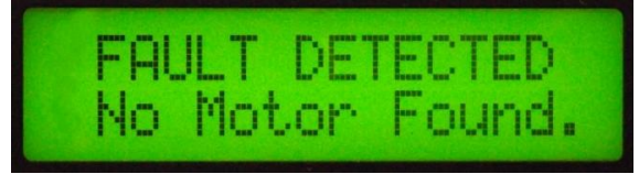
Display showing motor wiring fault
