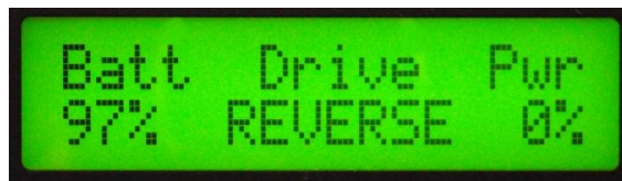
Direction switch set to Reverse
