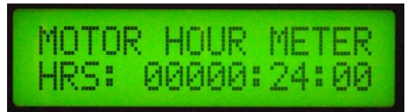
Display showing motor usage counter
