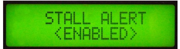
Display showing Stall Warning feature
