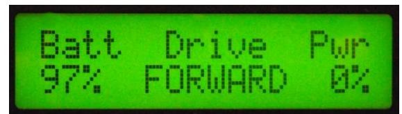
Direction switch set to Forward
