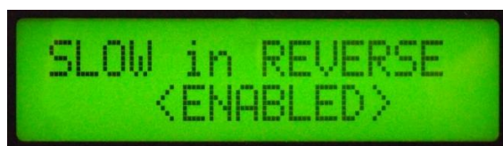
Setting up speed limiting in reverse
