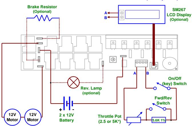
SM263 MODULE – ELECTRICAL CONNECTIONS (24V system)
