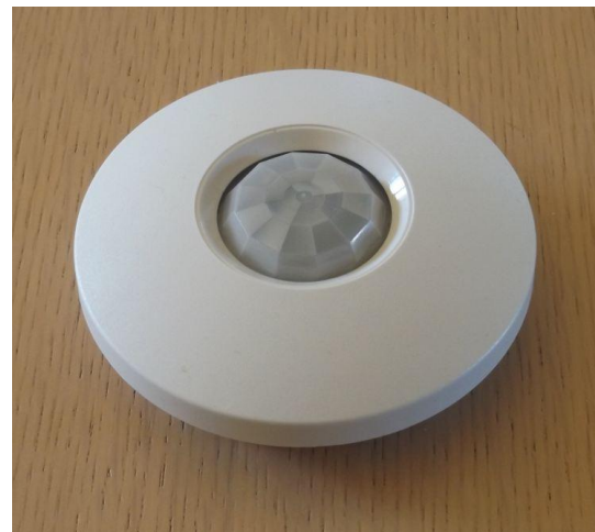
PIR sensor with cover in place
